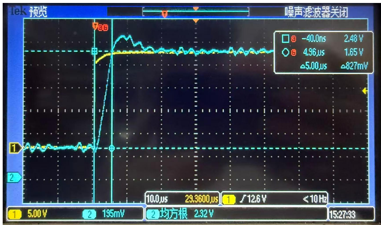
Fig.3 CH1 is primary magnetic field, and CH2 is output voltage; FFE-006F16T24JR series show output response time of 5 \mu s (~5 \mu s )
