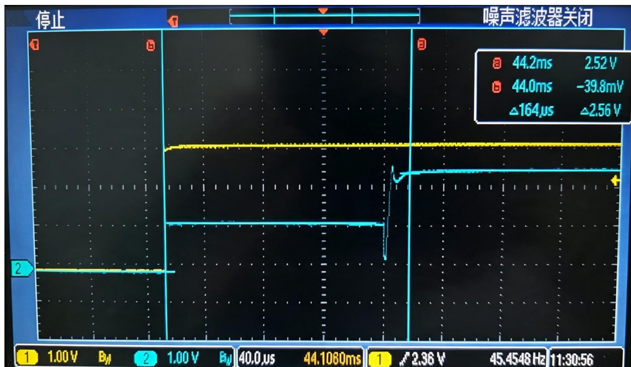
Fig.2 The yellow line of CH1 represents the Vcc power supply voltage, and the blue line of CH2 represents the Vout output voltage. The power-on response time of the FFE-006F16T24JR series is approximately 165 \mu s .
